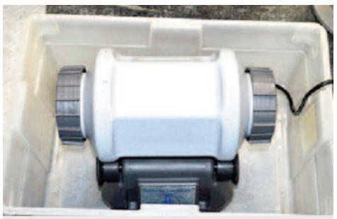
Photo 5. If you don't tighten the end caps sufficiently they can leak, so I put the tumbler in this big plastic tub just in case. It has not leaked.
