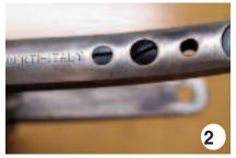
in until it just touches the mainspring. That way if additional tension on the mainspring is ever needed, the screw is in the gun and can be tightened a bit. Hint: when you are using the tension screw to adjust mainspring tension, first loosen the anchor screw a little. Tighten the tension screw and then retighten the anchor screw.
