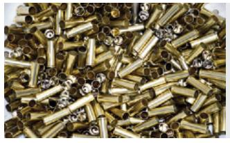
Photo 6. Brass after three hours of tumbling, then rinsing and drying.
