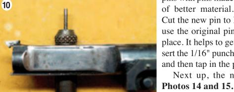
Cut the new pin to length, start the round end (or use the original pin) into the bolt and tap it into place. It helps to get everything aligned if you insert the 1/16" punch through the bolt and extractor and then tap in the pin, driving out the punch.
