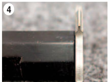
**Photo 5.** The smaller tip fits the lever screw, the receiver side screws and several other screws.
