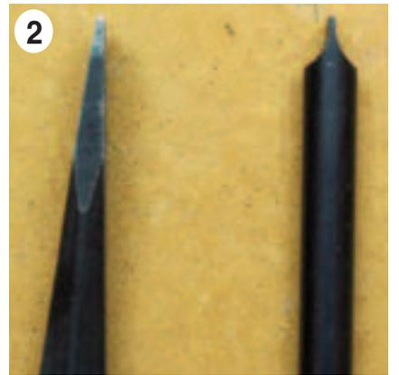
**Photo 2** shows a standard tapered screwdriver on the left and a hollow ground screwdriver on the right. The Winchester multi-tool is a hardened steel tool with two screwdrivers. It is flat and compact and has a hole in it so you can put it in your toolbox or carry it on a keychain.
